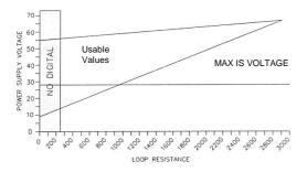
Digital communication requires a minimum loop resistance of 230 ohms.
