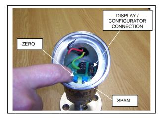
If more than just local Zero and Span is required, there is the unique D-CAL local display option.
