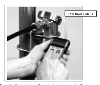
Once the first unit is configured, simply unplug the D-CAL unit and move onto the next unit.
